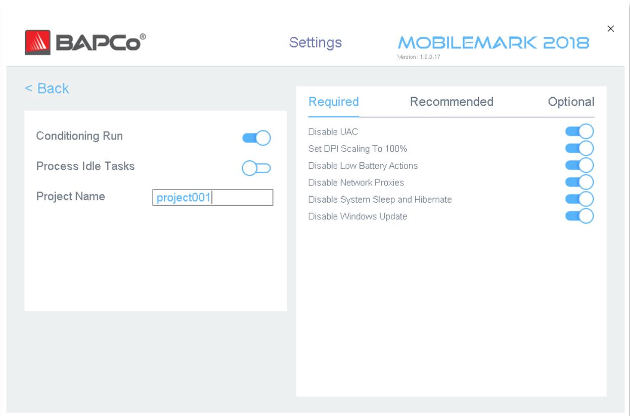
Figure 8: MobileMark 2018 configuration options on Windows 10
