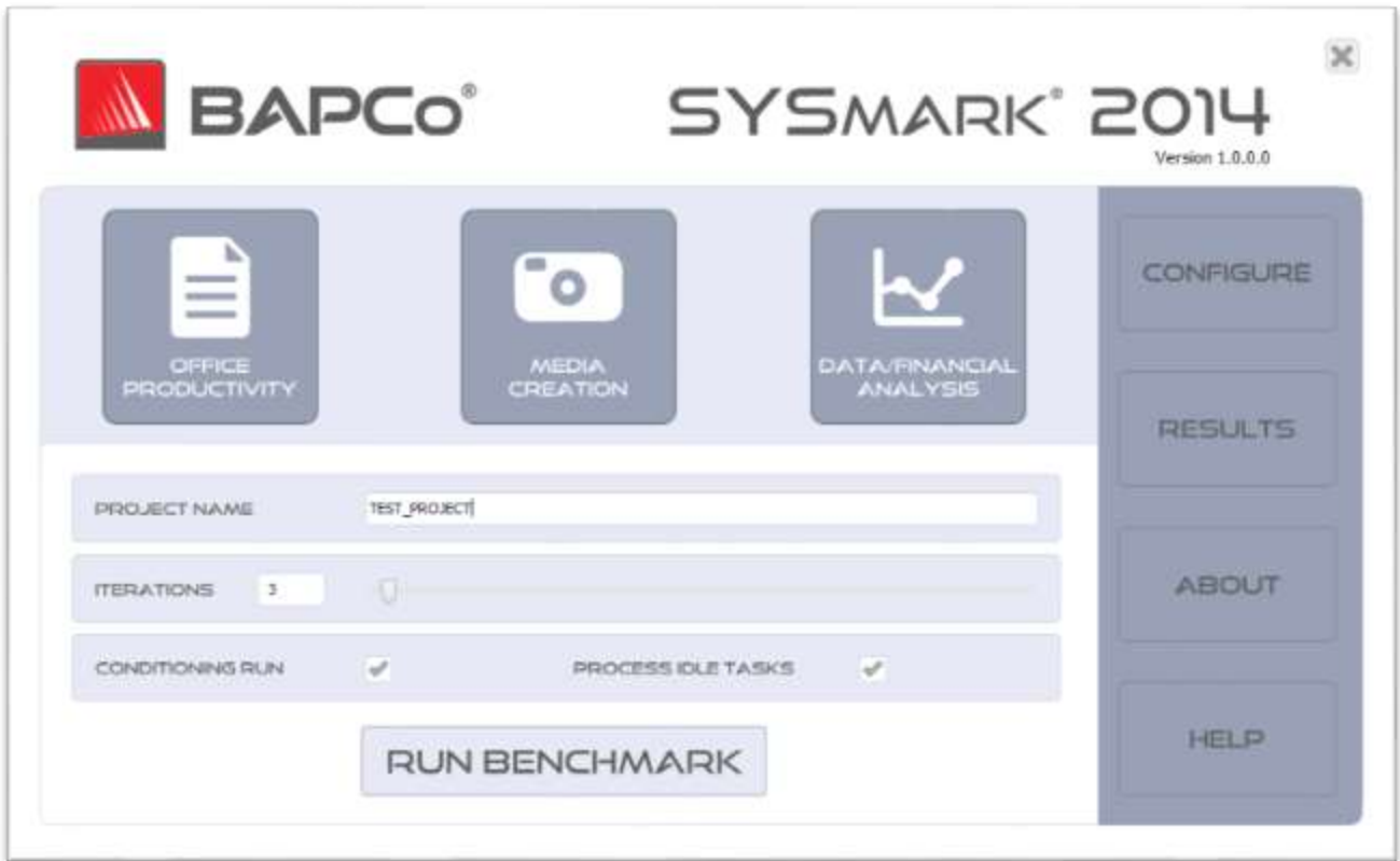
Figure 6: SYSmark 2014 interface shown with default scenario and iteration selections. Notice that the conditioning run is selected by default.
